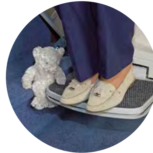
THE FOOTREST IS COVERED WITH NON-SLIP MATERIAL AND FITTED WITH SAFETY EDGES
